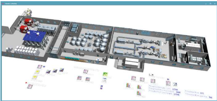
Fig. 2. Digital Model of the production in Tecnomatix Plant Simulation by Siemens
