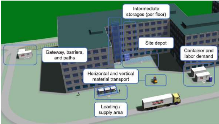
Fig. 4. 3D Plant Simulation model of an exemplary construction logistics layout
