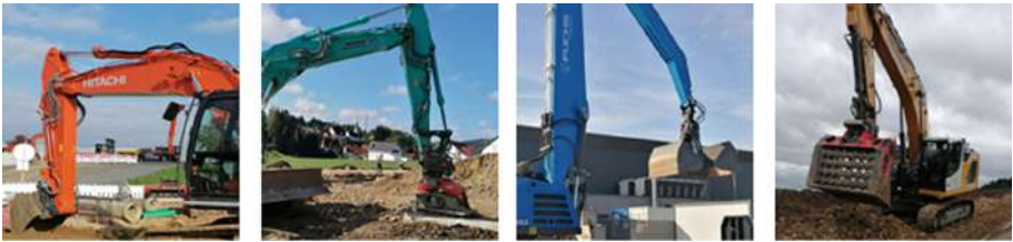
Fig. 1. Excavator attachments used in this work. From left to right: Bucket, compactor, grab and screener. Pictures taken by Marc Theobald.
