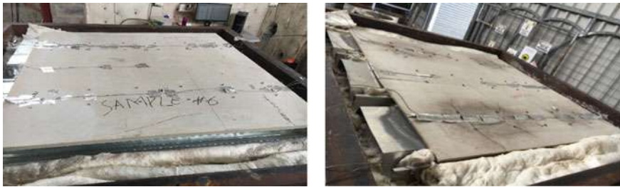
Fig. 7 a, b The fitting of the samples onto the furnace opening
