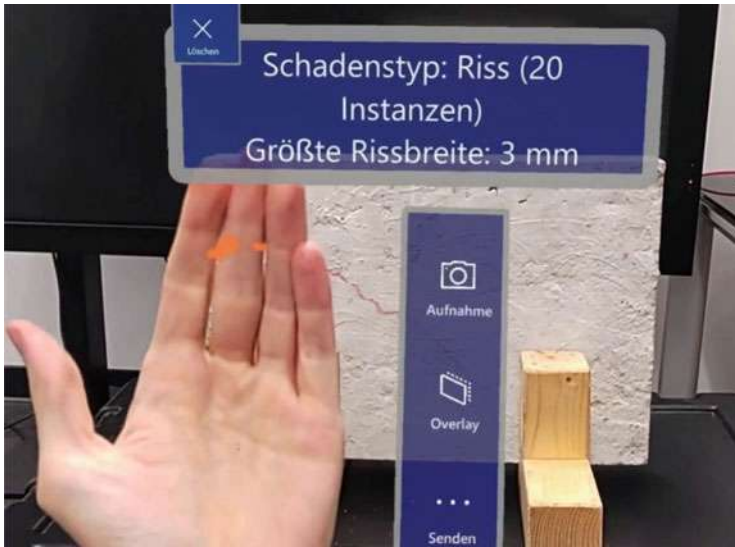
Fig. 6 Interface of the HoloLens 2 application. The functions for recording ('Aufnahme') and sending damage instances ('Senden') can be controlled through gestures and virtual interfaces. The crack in the concrete slab has been marked by the segmentation network in red.
