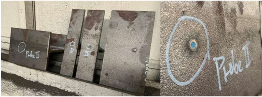
Fig. 1 Embedded passive RFID tags (rivTAG) in prefabricated steel structural profiles (Ed. Züblin AG)
