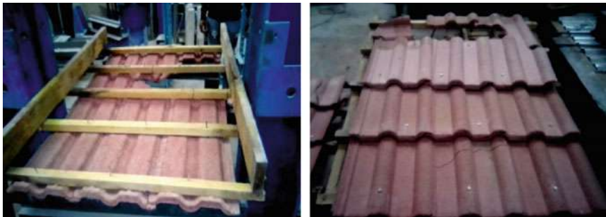
Fig. 8 Roofing tiles cracking and breaking in a row under the effect of applied uplift forces
