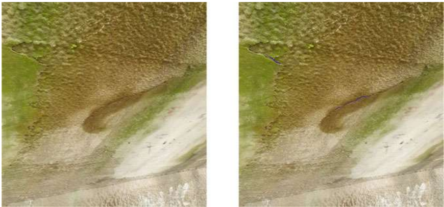
Fig. 10 False positive crack results with the FPN-Effb0 model. Blue color masks are crack predictions.
