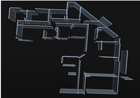
Figure 2: Automatic wall extraction in "EdgeWise". The set of detected walls is incomplete and contains wrong cuboids. Besides, the accuracy of wall dimensions is not perfect and a human needs to adjust wall length manually.
