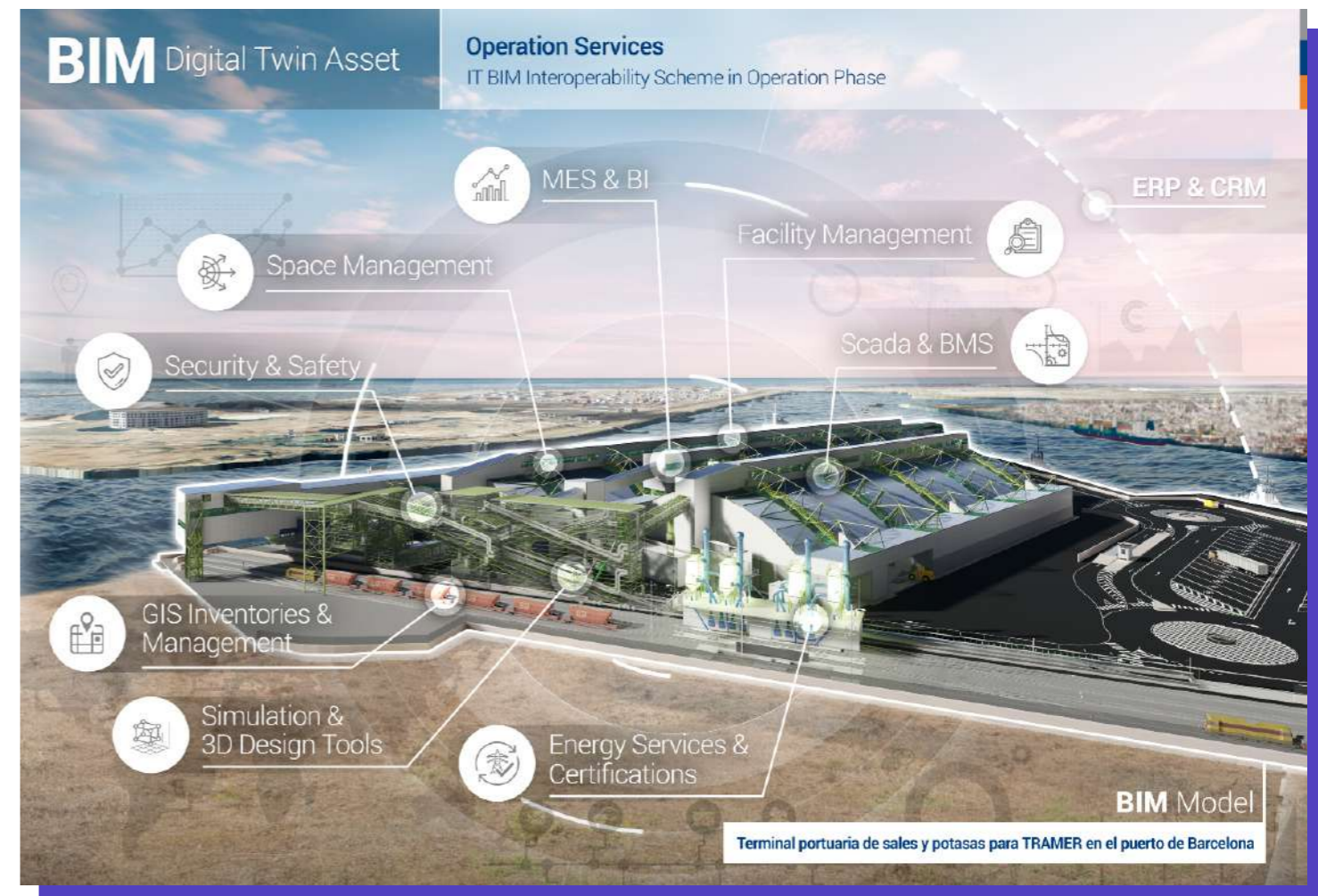
Conceptualisation of a Building Digital Twin Instance Interoperability Services (sketch by: M.Borràs)
