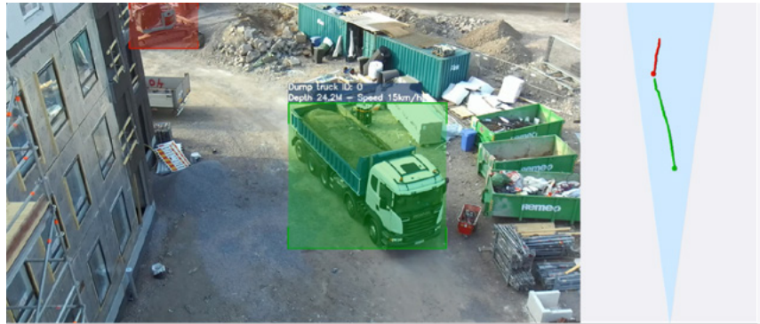
Figure 33. Dump trucks and excavators are recognised and tracked. The trajectories on the right are three-dimensional, shown from a bird's eye view.
